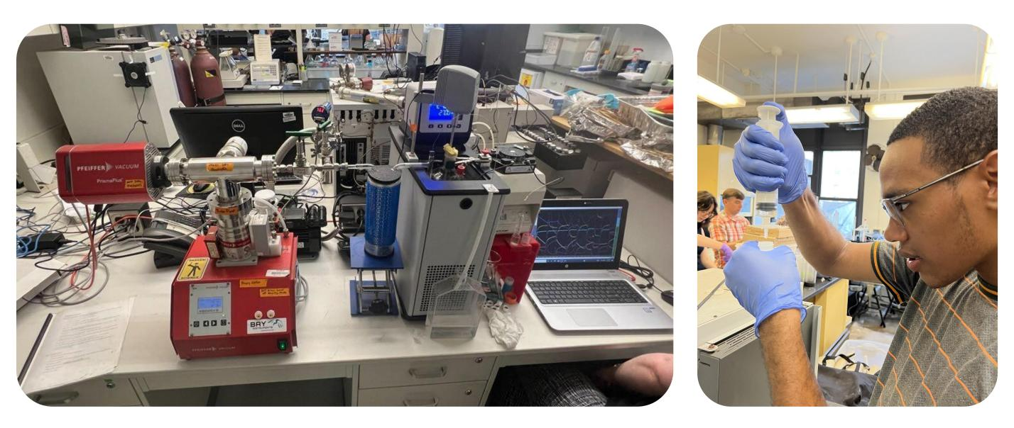
Water samples were collected from the cores in gas-tight vials and measured on a membrane-inlet mass spectrometer.
